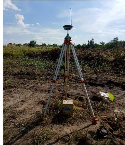
**Gambar 6.** Pengukuran base station
