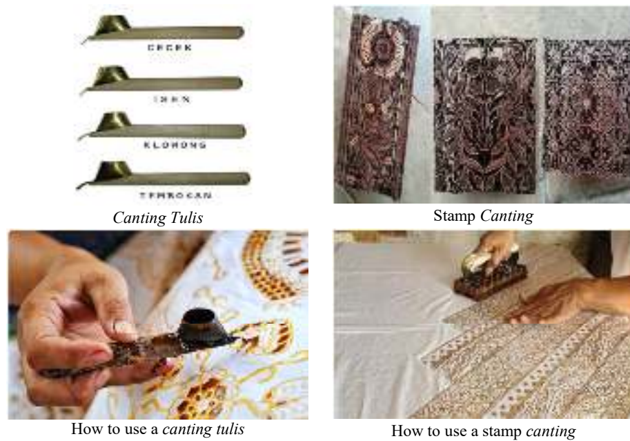
Fig. 1 Canting Tulis and Canting Cap and how to use them
