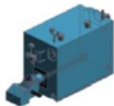
Gambar 12. Contoh 3D model LoD 400 (BIM Forum, 2015)
