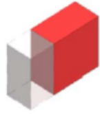
Gambar 9. Contoh 3D model LoD 100 (BIM Forum, 2015)
