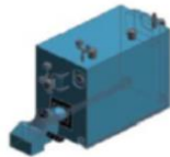
Gambar 11. Contoh 3D model LoD 300 (BIM Forum, 2015)
